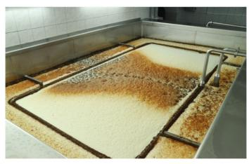
▲ Figure 21.3 A froth forming on the surface of the beer as yeast ferments the sugar to alcohol and carbon dioxide. The carbon dioxide in the froth prevents oxygen entering the mixture from the air – keeping conditions anaerobic.
