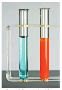
Figure 4.10b Glucose with Benedict's solution, before and after heating
