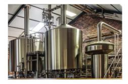
A **fermenter** is any vessel that is used to grow microorganisms used for fermentation. Even a baking tray containing a ball of dough could be defined as a fermenter!
