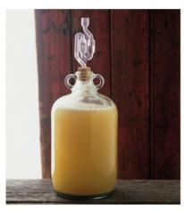
Figure 21.2 A small fermenter for producing homemade wine. The U-shaped tube at the top is a water-filled airlock that prevents oxygen entering the fermenter but allows carbon dioxide to escape.
